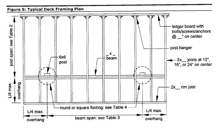
Each joist shall be attached to the beam as shown in Figure 6. Joists may bear on and overhang past the beam a maximum of L/4. Use Option 1 or Option 2 to attach the joist to the beam. Option 1 shall only be used if the deck is attached to the house with a ledger (see LEDGER ATTACHMENT REQUIREMENTS) or as
